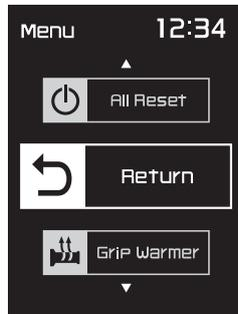
2. Push the "MENU" switch to exit the setting mode and return to the standard display mode.
