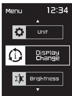
2. Push the “MENU” switch, use the select switch to highlight the display to change, and then push the “MENU” switch again.
