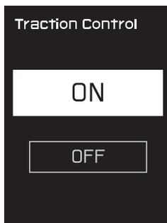
3. To set the traction control system to "OFF", push the select switch "∨" side for 2 seconds.
